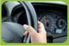
Alternatively, turning the steering wheel just after moving off will give an immediate indication that the power assistance is functioning.
