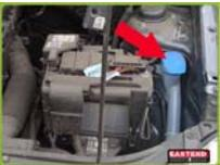
**Q** Open the bonnet, identify where the brake fluid reservoir is, and tell me how you would check that you have a safe level of hydraulic brake fluid.
